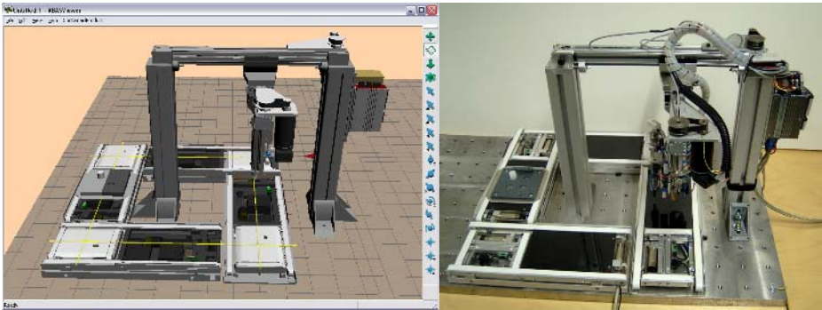
Fig. 2. A 3D view of a system built by intelligent physical agents (ABAS Viewer) and the correspondent physical implementation
