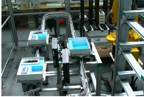
Fig. 2. The empty box on the right hand side of this loop (sub-loop 1) corresponds to a kanban that is waiting to be fulfilled
